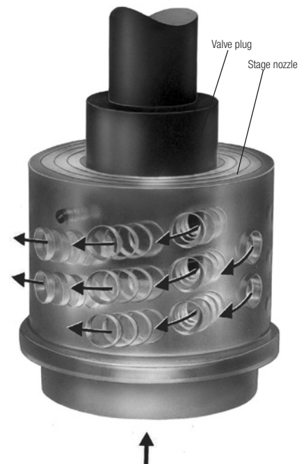
Flow through ZK 29 radial stage nozzle
