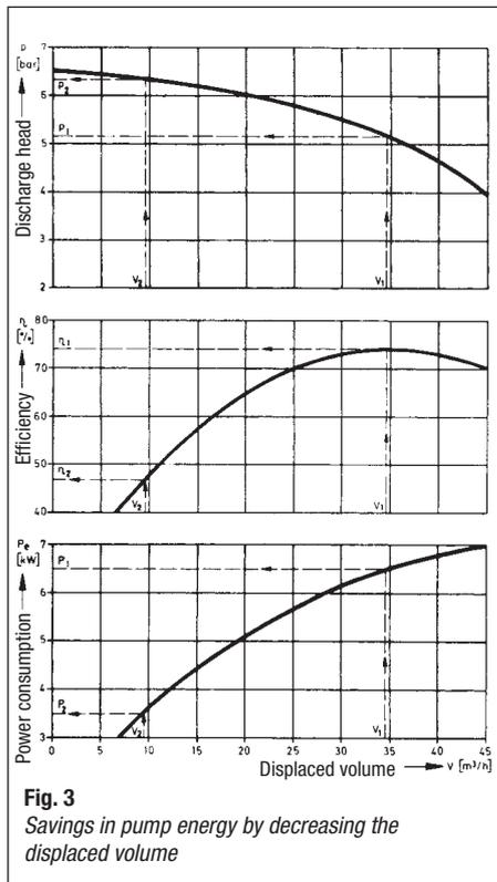
Despite the reduced pump efficiency (see second chart, Fig. 2), 46.2 % of pump energy are saved.
