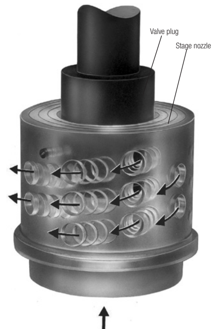
Flow through ZK 29 radial stage nozzle
