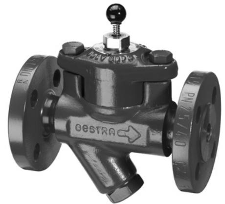
the closing pressure to which the AK 45 has been adjusted, the valve closes automatically. The closing pressure is set at our works to 0.8 bar. When the pressure in the system drops again, the valve opens at approximately the same pressure required to close the valve, i. e. opening pressure  $\approx$  closing pressure.
