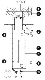
**Fig. 4** Protection tube for installation of electrode inside the boiler
